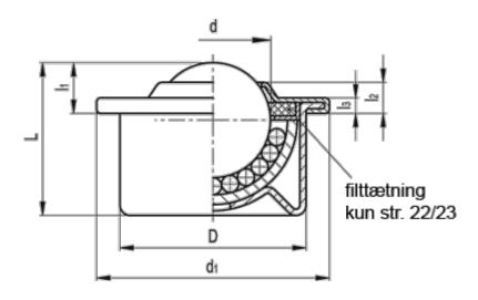
$$\begin{array}{lll} d & = 22.2 \\ D & = 36 \\ d1 & = 45 \\ L + / - 0.3 & = 29.5 \\ I1 + / - 0.3 & = 10.0 \\ I2 + / - 0.3 & = 6 \\ I3 & = 3.0 \\ Max load (N) = 900 \end{array}$$
